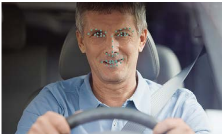
The position of the 49 reference points is determined using the Kostal image recognition software.
