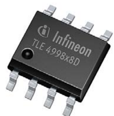
Dual Hall sensor as packaged component
